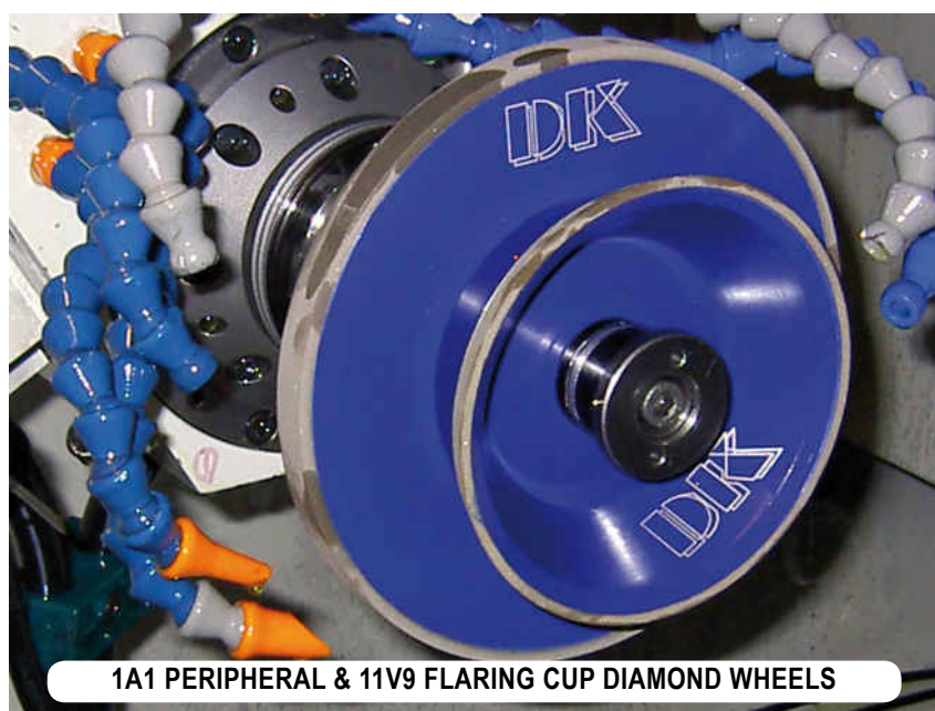
RESIN DIAMOND WHEELS ON AN ANCA CNC MACHINE
